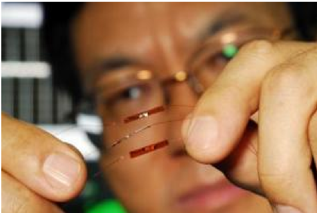
Georgia Tech Professor Zhong Lin Wang holds a prototype flexible charge pump. The device generates alternating current as zinc oxide wires are stretched and then released. (Credit: Georgia Tech Photo: Gary Meek)
